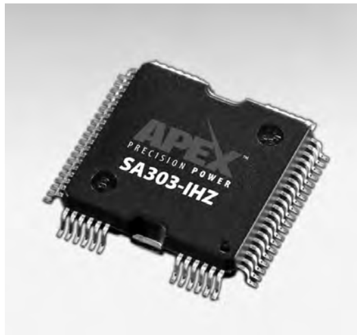
Figure 2. 64-Pin QFP, Package Style HQ
