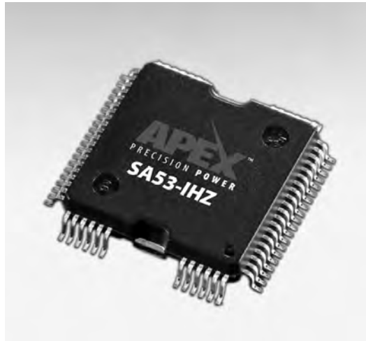
FIGURE 2. 64-pin QFP, Package Style HQ
