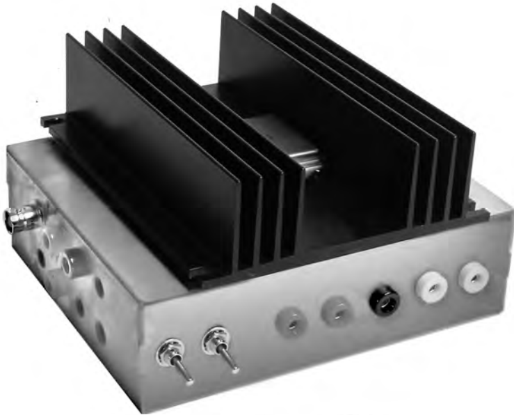
Figure 2. External with heatsink (heatsink, amplifier, connectors and switches not supplied).
