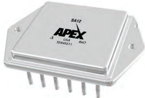
12-PIN POWER DIP PACKAGE STYLE CR
