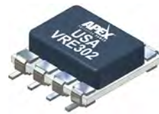
8-pin Surface Mount Package Style GD
