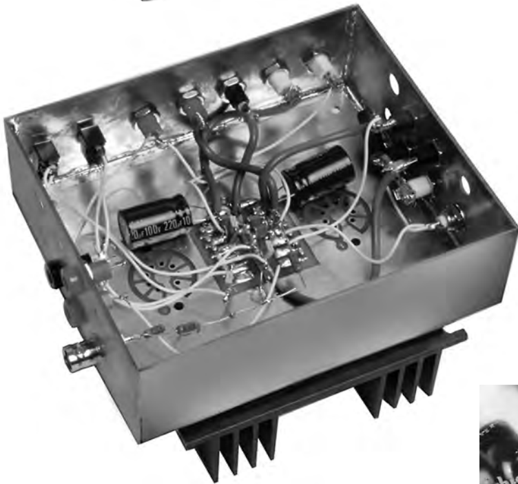
Figure 3. Inside of assembled box. Holes for components on long side were user drilled.
